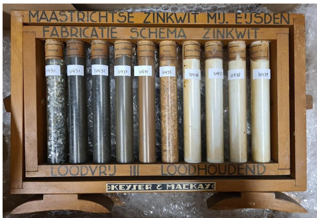
Figure 1: Samples from the production process of zinc white at the Maatrichtse Mij. Eijssen.
